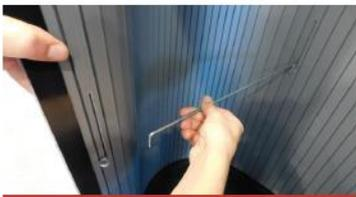
4. Place the hook between the 2 pins on the left side, connecting them together.
